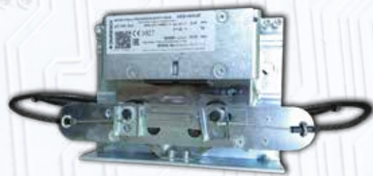
Bidirectional e-ASG UD WRA safety gear with double coil solenoid and remote tripping A single solenoid to trip the 4 locking rollers
